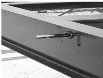
Fig. 1-Through Frame Crank Extension w/pin
