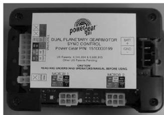
Fig.1 Slideout Controller
