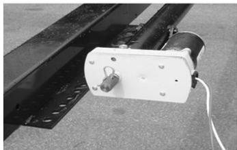
Fig. 3-Hex Head Crank Extension
