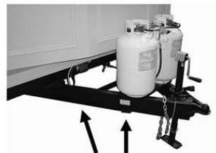
Electrical wiring & safety break-a-way switch
